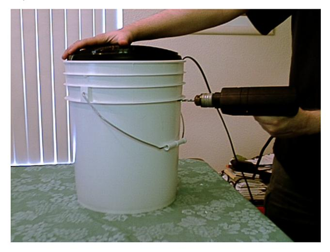
Step 4: Drill about 8 or 10 holes around the bucket.
